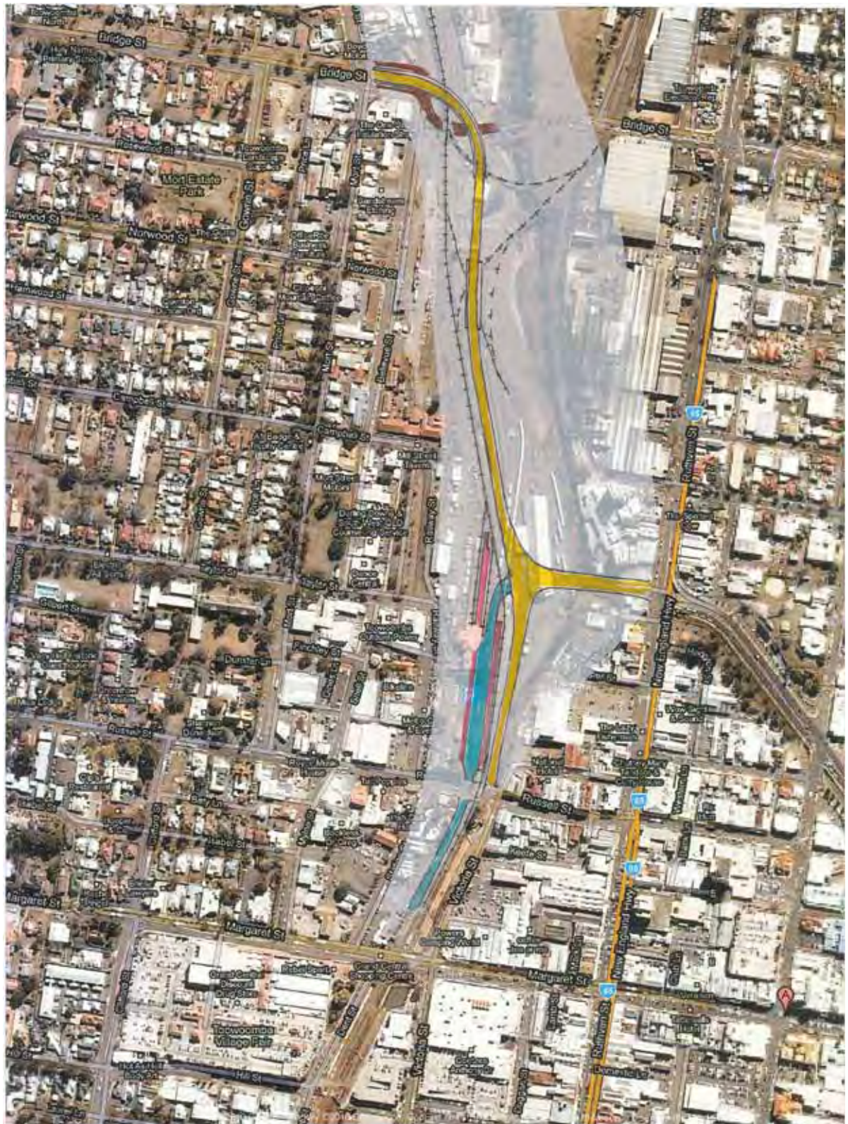
Figure 6.1 – Proposed Toowoomba Railway Station Bus/Rail Interchange
