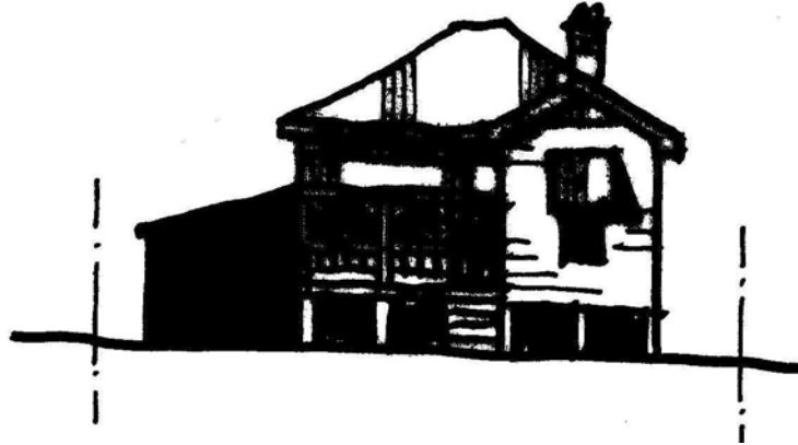
NOT RECOMMENDED Attached Lean-To
