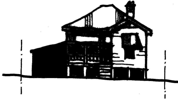
NOT RECOMMENDED Attached Lean-To
